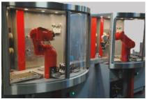
PR/TX60 OPTIONALS Automatic tray loading Unloading device for 6 trays Double polishing configuration for outside and inside ring polishing : Both units PR/TX60 I and PR/TX60 O are installed in line and connected with each other by a conveyor belt. Both units are extra equipped with a tray loading and unloading device. This configuration increases the production speed by 2!
