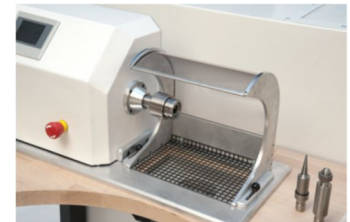
Polishing motor block with quick change feature for different buff holders
