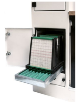
Filtering chamber with double filter and dust recovery drawer
