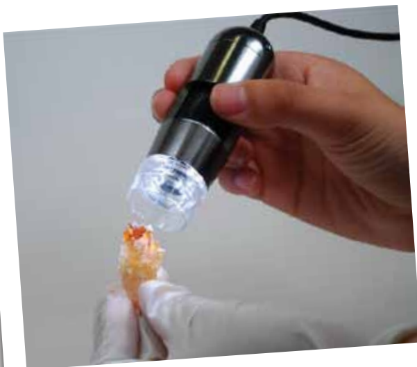
Inspection of gemstone with Dino-Lite
